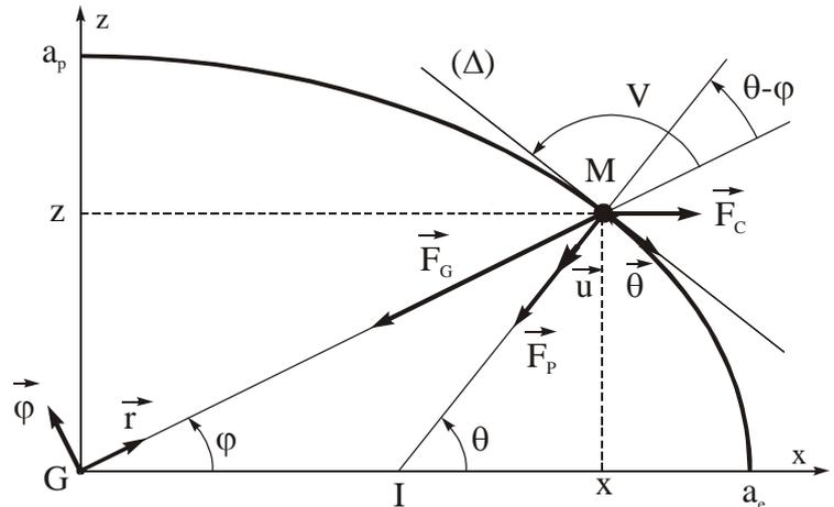
$$(I) \quad \begin{cases} F_p = g = \frac{\partial U}{\partial r} \cos(\theta - \varphi) + \frac{1}{r} \frac{\partial U}{\partial \varphi} \sin(\theta - \varphi) - \omega^2 \cdot r \cdot \cos \varphi \cdot \cos \theta \\ 0 = \frac{\partial U}{\partial r} \sin(\theta - \varphi) - \frac{1}{r} \frac{\partial U}{\partial \varphi} \cos(\theta - \varphi) - \omega^2 \cdot r \cdot \sin \varphi \cdot \cos \theta \end{cases}$$
